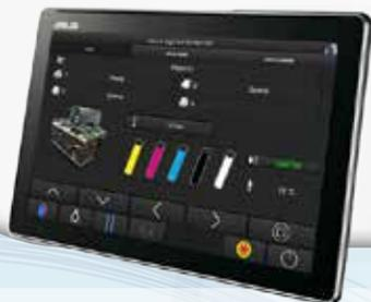
The printer remote management via tablet allows you to get an overview of the printer status and be able to perform routine management tasks without the need to physically visit the printer.
